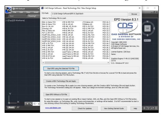
You may pick **Open without a TCH File** button or press **<ESC>** to bypass and continue the first loading of the EPD Environment.
